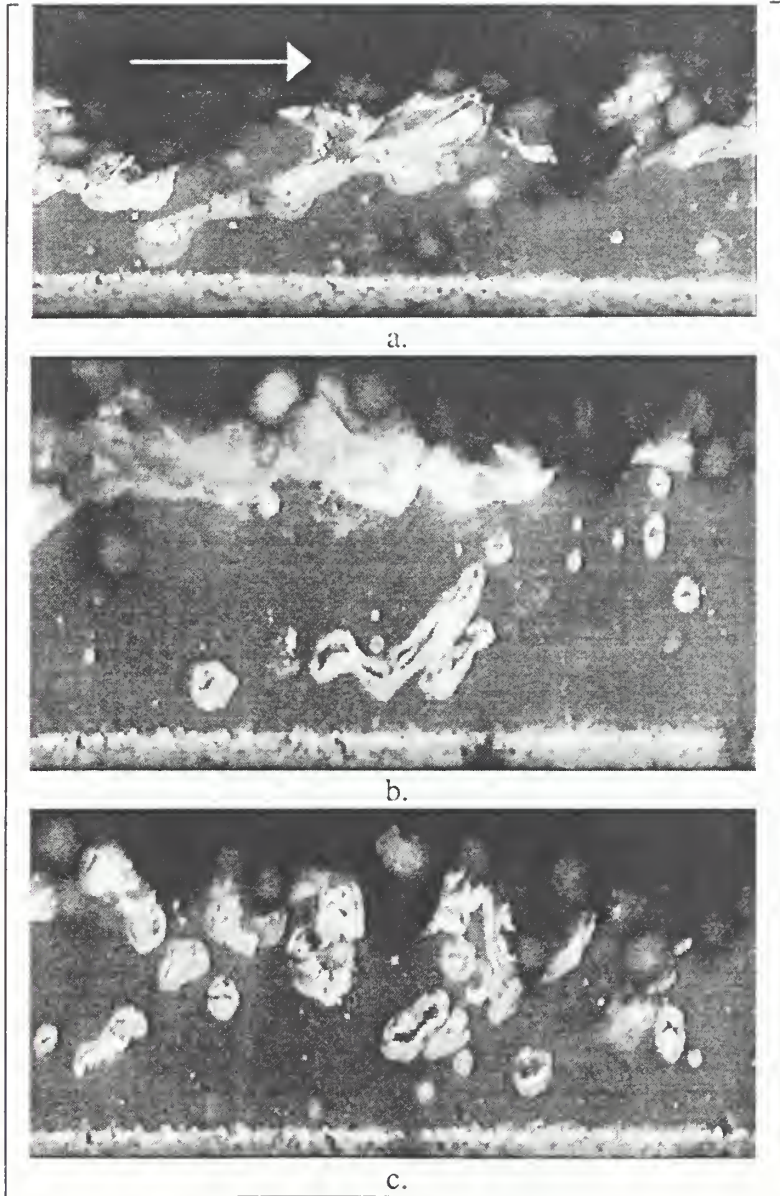
Figure 62. Photographs of the interior of a rough-wall liquid jet formed in the recirculating water tunnel. Re_x = 2.3 \times 10^6 , Re = 2.8 \times 10^4 , Fr = 9 , We = 1100 , k/ho = 0.08 .
